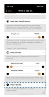
NOTE: The TRED must be unpaired to change the profile. To unpair, double tap the TRED in the network and scroll to the bottom of the options to "Unpair Device", then follow step on from Step 1 above.
