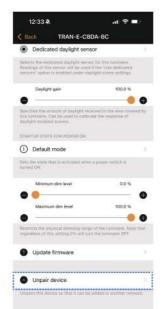
NOTE: The TRAN must be unpaired to change the profile. To unpair, double tap the TRAN-E-CBDA-BC in the network and scroll to the bottom of the options to "Unpair Device", then follow step on from Step 1 above.
